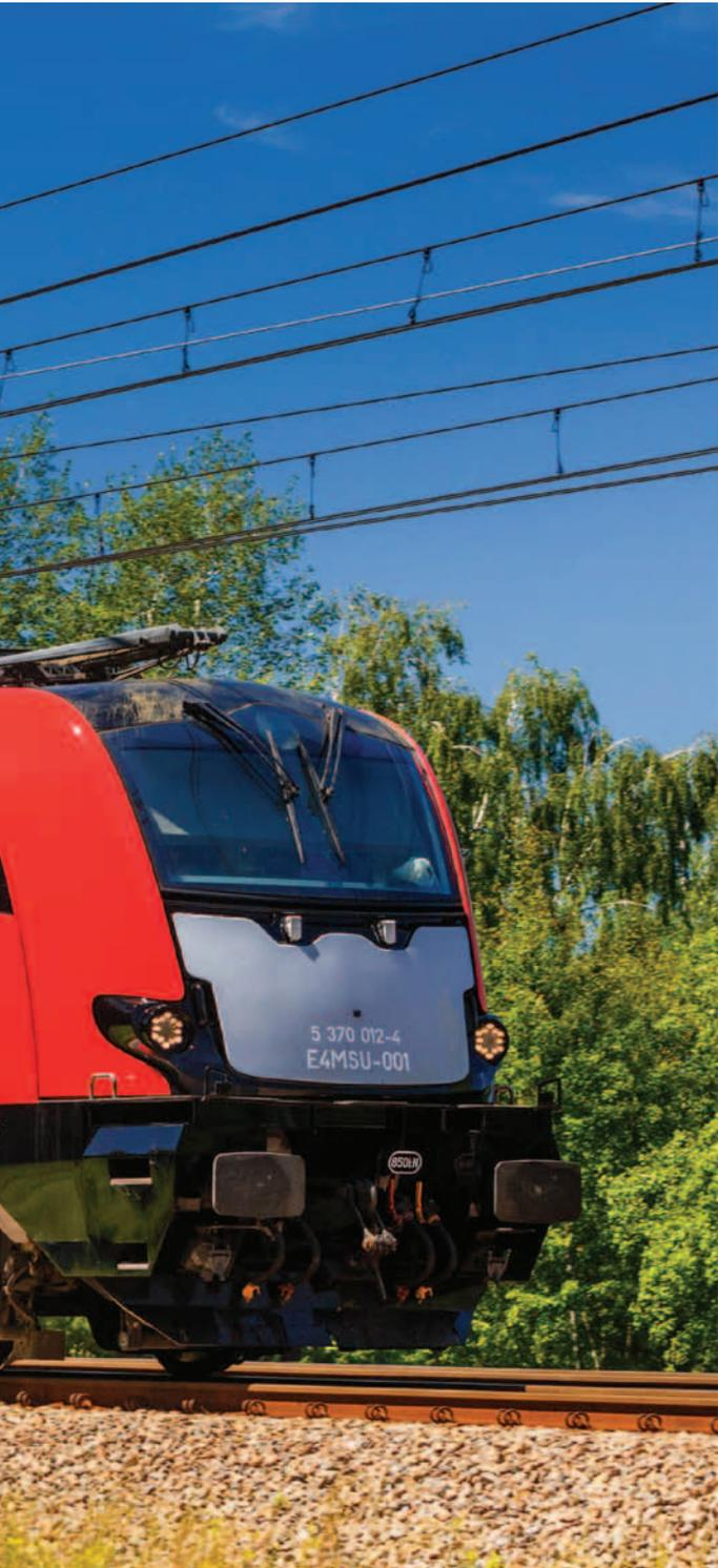
Griffin is a universal family of four-axle locomotives designed for pulling freight and passenger trains. It is the first Polish multisystem locomotive adapter to be used both with the 3 kV direct current power supply system and 15 kV or 25 kV alternating current power supply systems.
